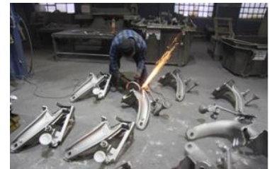
Figure 10: Workers had to manually cut the castings for many product variations. With HORSE, the task is now automated, and workers can be more focused on the final product quality.
