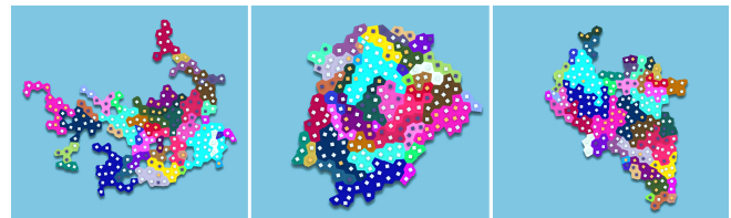
Figure 6. (left) A minimal cohesion factor leads to very rugged islands with many holes. (middle) A very high cohesion factor reduces holes greatly and creates compact islands. (right) Our dynamic cohesion factor, combined with the claiming of large regions first, the island preserves some of the ruggedness, yet it minimizes holes.
