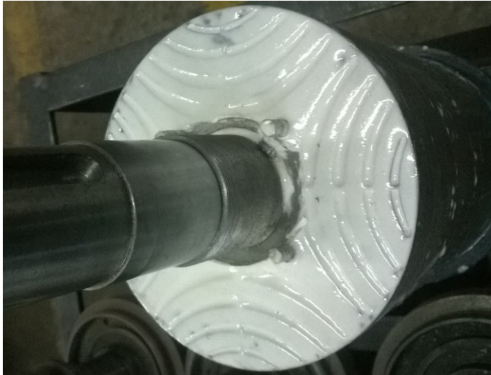
Figure 5.29. The prototype's rotor after injection of the Epoxy adhesive.
