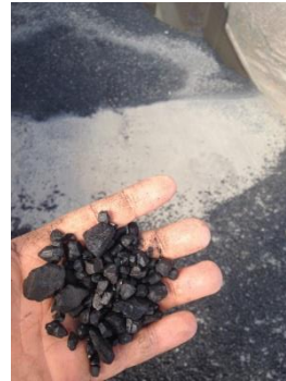
Figure 1 'good coal' being rejected by MPS mills. Raw coal, much larger than pictured, is getting stuck in the pyrites removal system, therefore calling for a size upgrade
