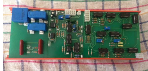
Figure: 1 – Four Quadrant STATCOM Inverter
