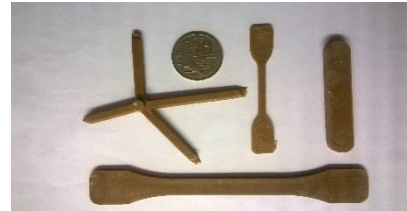
Figure 1 shows the hemp/PP reinforced composite after extrusion/injection method. A 20cent coin is placed near the samples.
