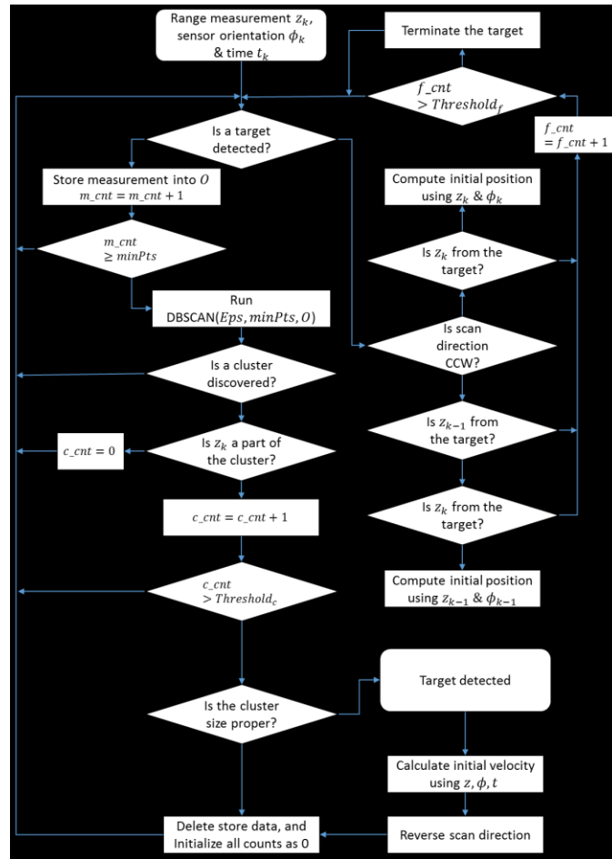
Figure 11. Flowchart of the proposed target detection algorithm with computing the initial conditions of target position and velocity
