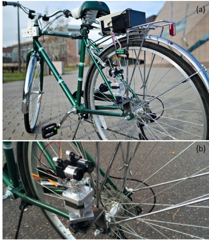
Figure 9. Laser sensor system on bicycle. (a) Rear-facing sensor. (b) Zoomed in.
