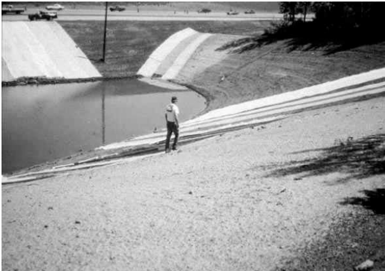
Mn/DOT and the University created an erosion control test site to test and compare products.
