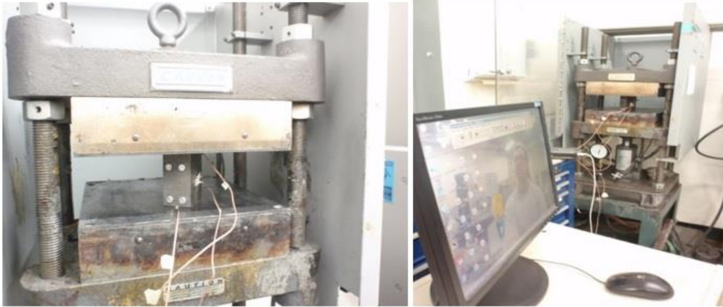
Figure 3.5. Different thermometers were installed to control the temperature of compacted powders.
