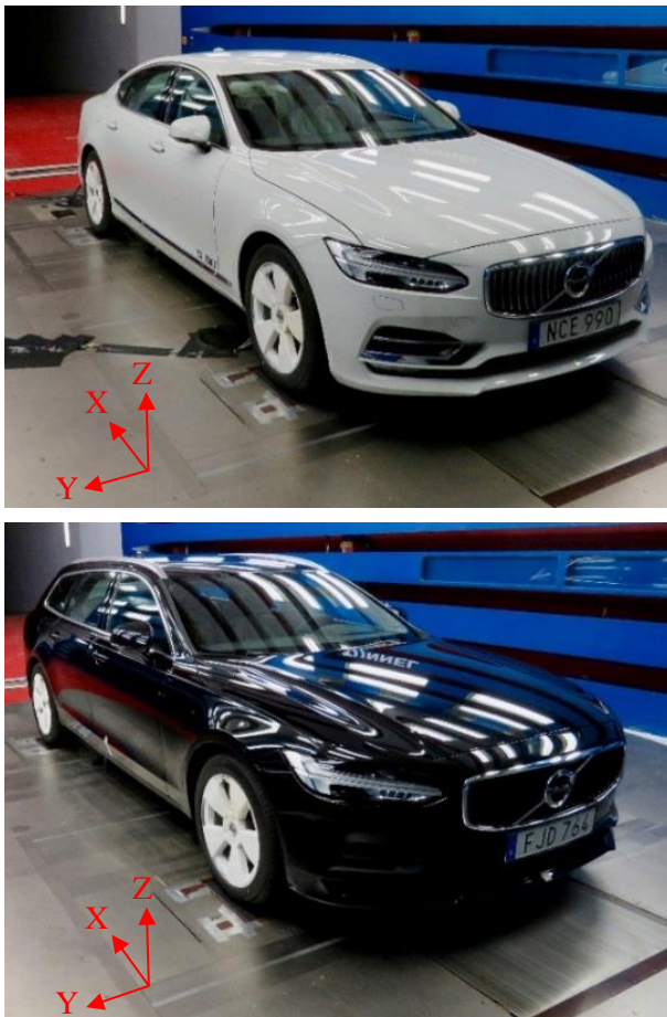
Figure 1. The test objects. Upper image is the sedan vehicle (Volvo S90), and below is the estate vehicle (Volvo V90). Coordinate system shown.
