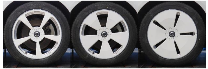
Figure 5. Rim configurations used to separately investigate the coverage area at 40 %, 65 % and 90 % coverage.
