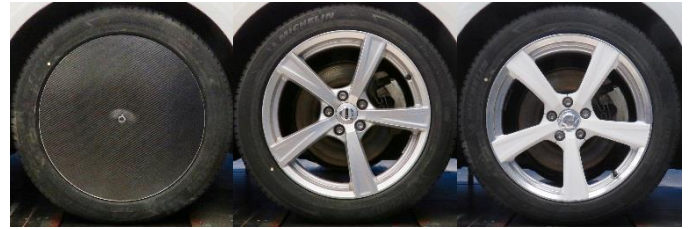
Figure 4. Rim configurations used to evaluate the modular wheel concept: a covered wheel (left), a production wheel (middle) and a representation of production wheel (S19) using the modular wheel concept (right).
