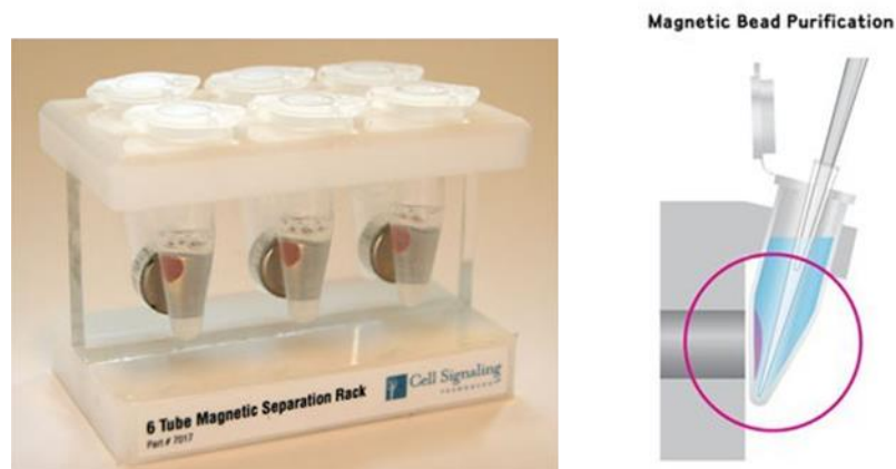
Figure 30 - (Top) Scheme of immunoprecipitation procedure. (Bottom) Representative image of a magnetic rack, as well as sample purification by bead assembly at the magnet and removal of supernatant. Images taken and compiled from websites of Rockland Immunochemicals, Cell Signaling and Fisher Scientific.
