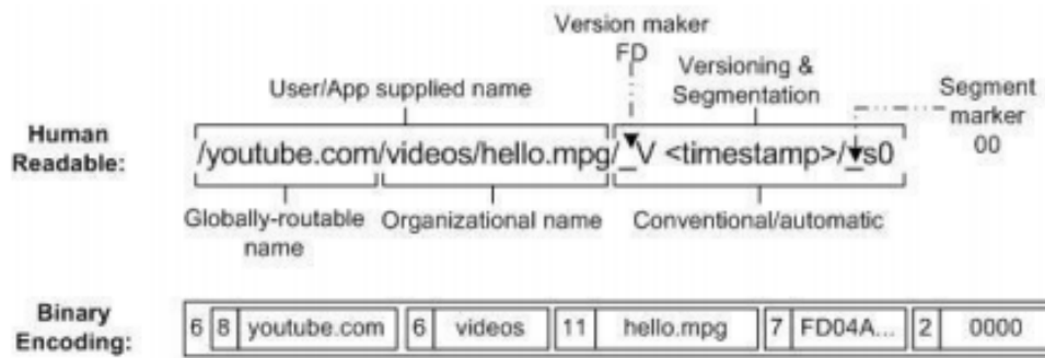
Figure 2. 3 The Hierarchical and Human-Readable Naming Scheme with Binary Encoding Format in NDN [3]
