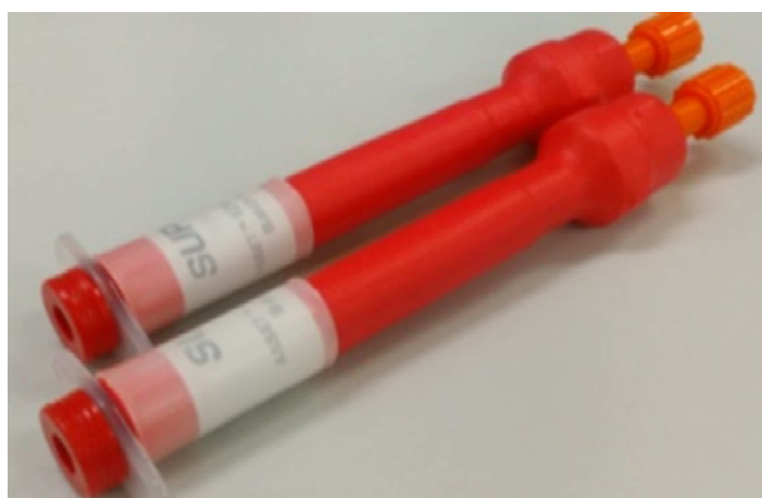
Fig. 2-10 Tubes for determination of HNCO concentration. (ASSET™ EZ4-NCO Dry Sampler by Sigma-Aldrich)
