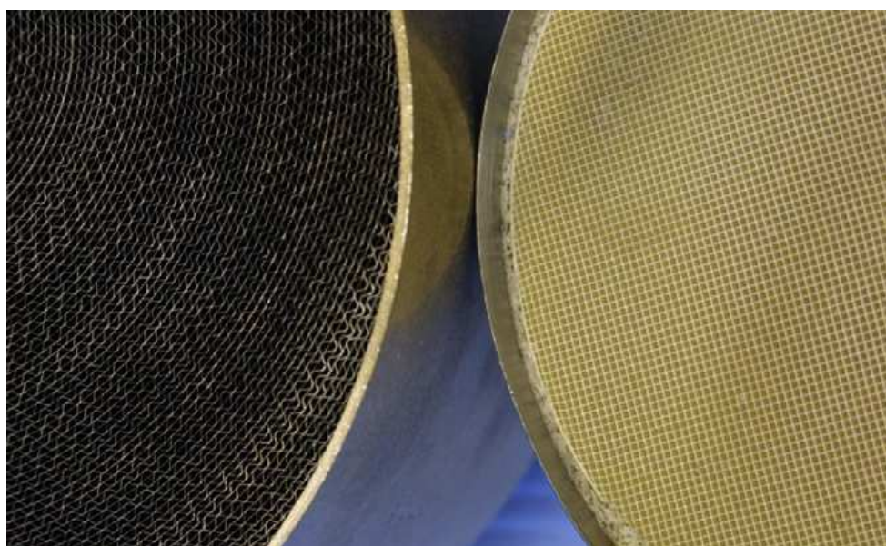
Fig. 1-4 Typical examples of a metal foil catalyst substrate (left) and an extruded cordierite substrate (right). (15)
