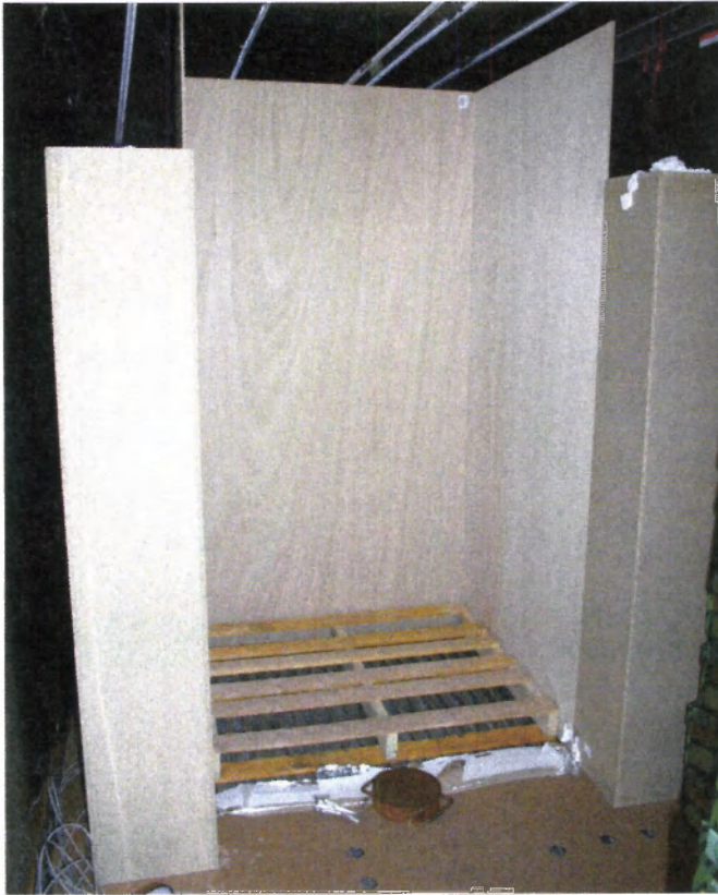
Figure 5 Box that guides air through the pallet
