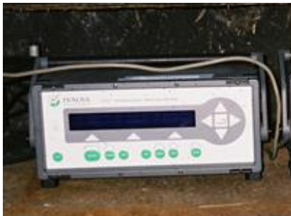
Figure 7 Infrared photoacoustic monitor for CO 2 concentration measurements.
