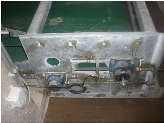
V-shaped manure belt. Top left: collection area of urine and faeces. Top right: manure belt underneath slatted floor. Below: operating mechanism.
