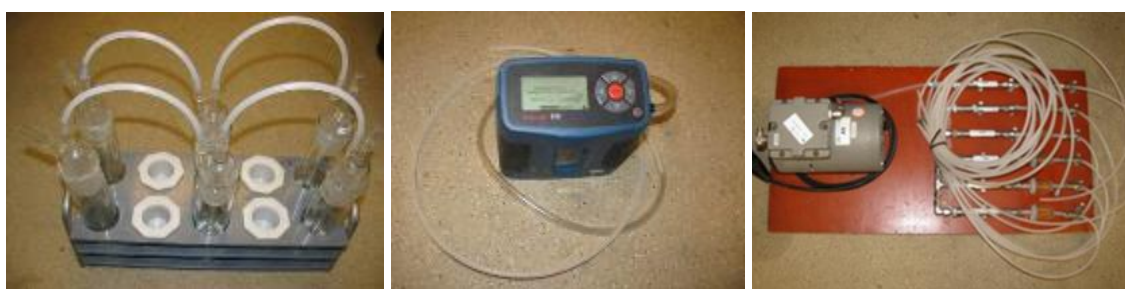
Figure 3 Measurement method for ammonia concentration measurements. Left: acid traps; Middle: flow meter; Right: pump.
