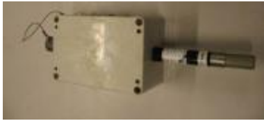
Figure 6 Rotronic for temperature and relative humidity measurements.
