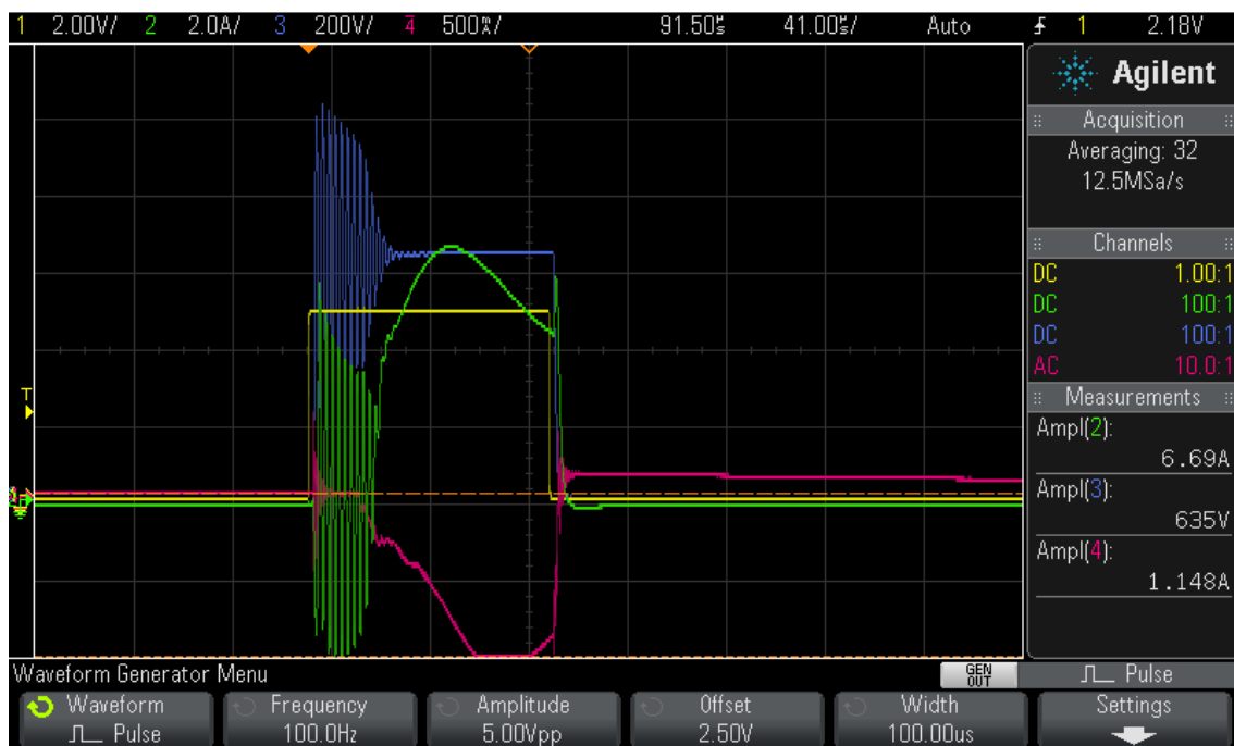
Figure 4-1: The HiPIMS voltage, current waveforms used for the SnO x thin film deposition.
