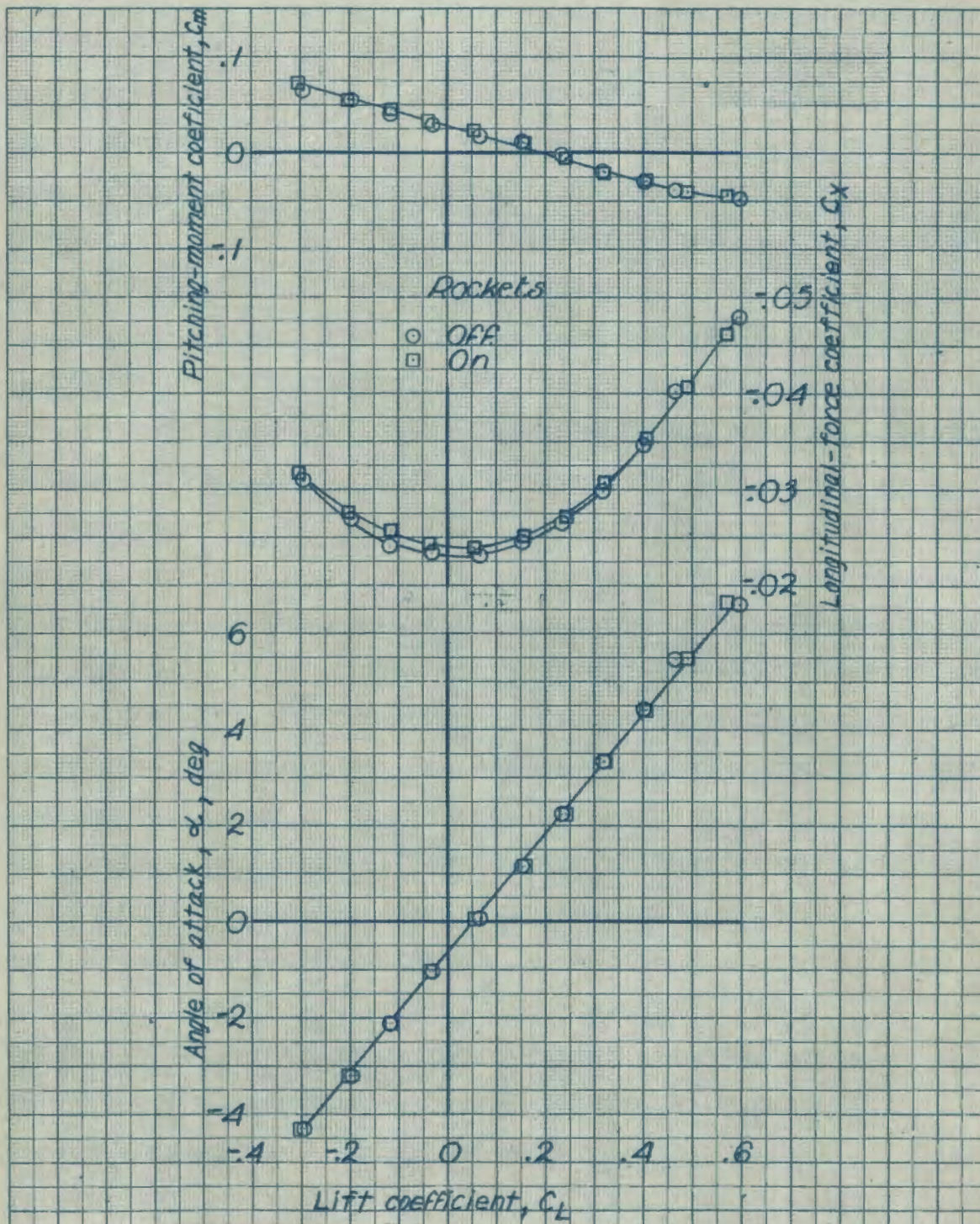
Figure 32.- Effect of rockets on the aerodynamic characteristics in pitch of the 1/5-scale model of the Republic XP-84 airplane with revised horizontal tail. \delta ding power; cruising configuration; i_t = 0^\circ .
