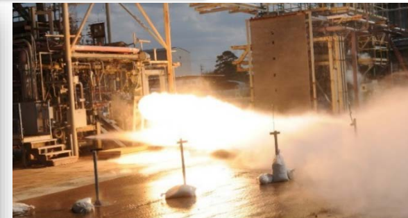
Ox-Rich Staged Combustion Subscale Main Injector Testing of 3D-Printed Faceplate
