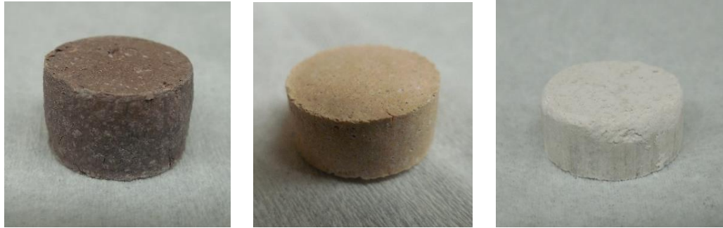
Figure 2. Bioactive glass cm size pellets after annealing at 200 °C. From left to right: UMBG1, UMBG2, and UMBG3.
