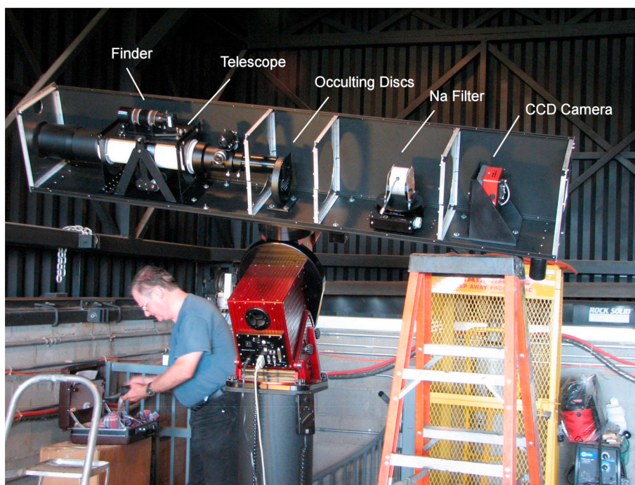
Fig. A2. Coronagraph with cover removed showing the layout. Roy Tucker is shown assembling the coronagraph.
