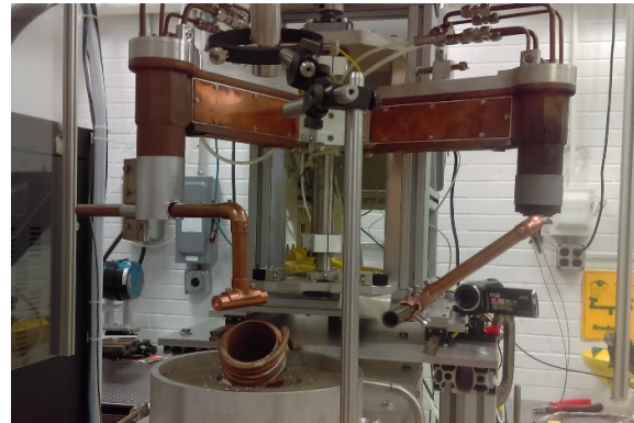
Figure 1. Image of torch facility including inert gas shroud, flow diverter, and probe and test article mounting hardware.
