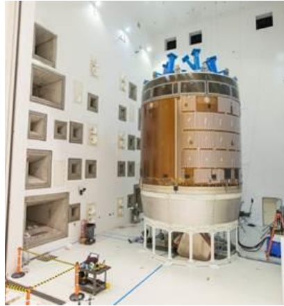
ESA's Structural Test Article testing in NASA's acoustic test facility at NASA PBS. Credit: ESA
