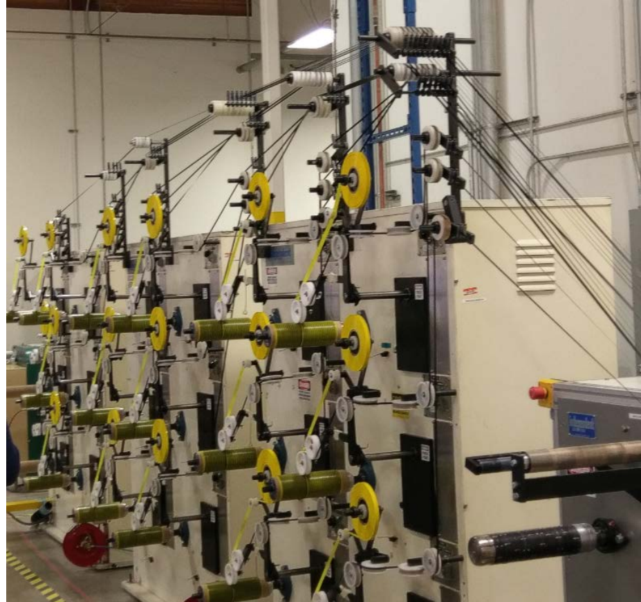
Tape slitting: extra steps to take 305mm (12") wide material to 6mm (1/4") wide
