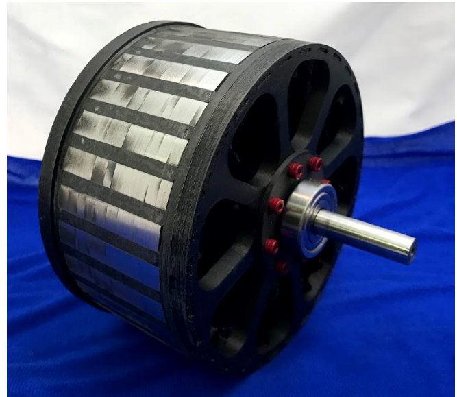
Fig. 11. PT-2 sun gear and modulator subassembly ready for assembly with ring gear, with dark lines on modulator pole pieces showing where separations occurred in wire EDM cutting process.
