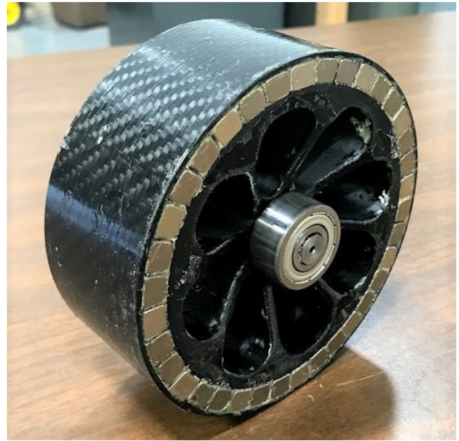
Fig. 6. PT-2 sun rotor sub-assembly including fully cured magnetic array, carbon fiber retaining hoop, high speed shaft, and bearing.
