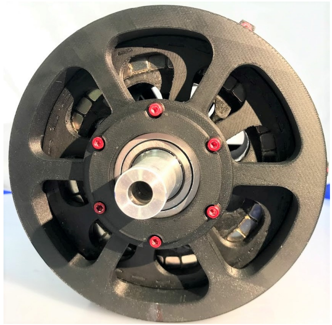
Fig. 13. PT-2 fully assembled with the axial face of the sun gear magnets visible through the modulator and ring gear caps.
