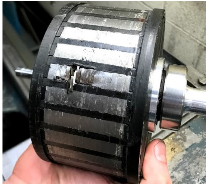
Fig. 19. PT-2 second modulator with sun gear still inside after testing resulted in a broken pole piece.
