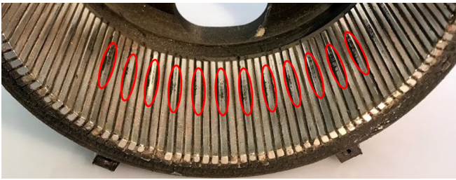
Fig. 15. Ring gear after contact had occurred showing marking compound on every third magnet examples of which are circled in red.
