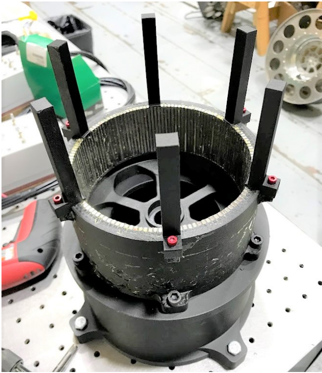
Fig. 12. Ring gear bolted to a bench-top with six guide-ways attached to its top ready for assembly with sun-modulator sub-assembly.
