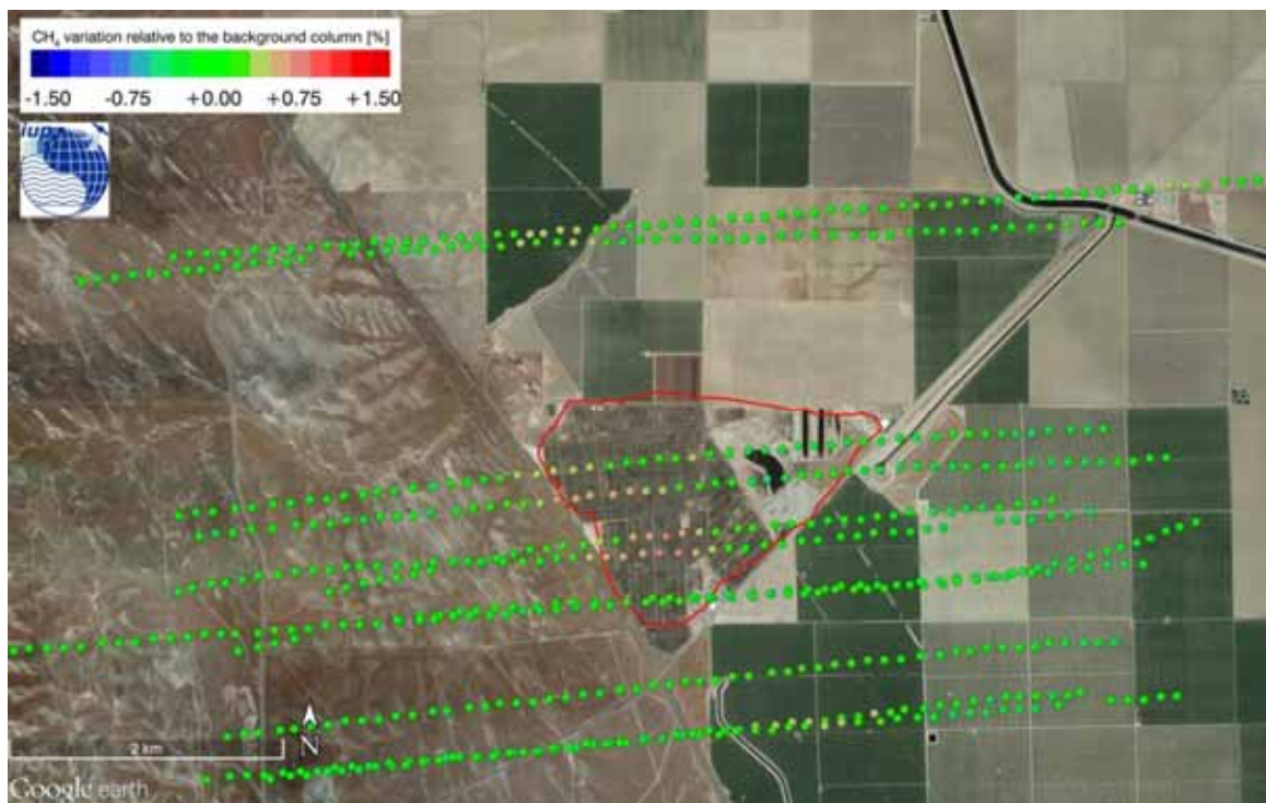
Figure 73: Normalized column averaged dry air mole fraction of CH_4 of the MAMAP remote sensing sounding of Harris Ranch (encircled by the red solid line) on 2014-05-30.
