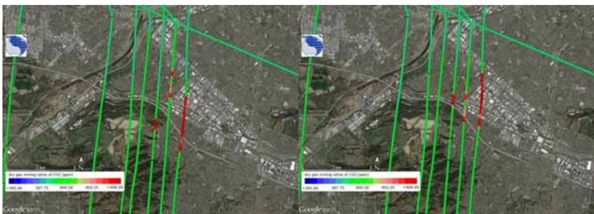
Figure 25: Picarro in-situ measurements of CO_2 at remote sensing altitude over the Puente Hills Landfill on 2014-06-12. Left: Original data set. Right: By 16 s corrected data set.
