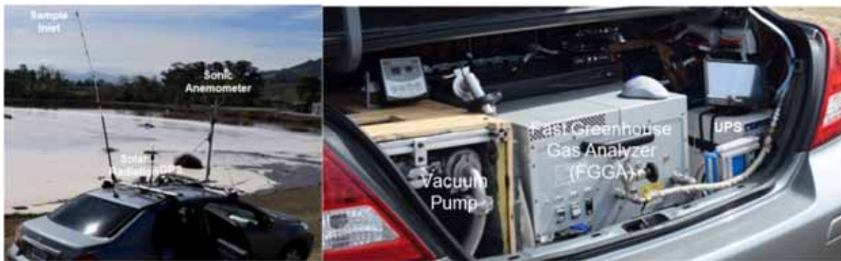
Figure 10: AMOG Surveyor images at the California State University Polytechnic Dairy waste pool showing roof and trunk packages.
