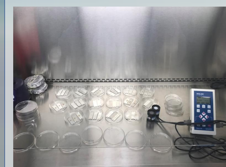
Figure 5. Radiometer and sample setup in the BSC prior to turning on the UV light.
