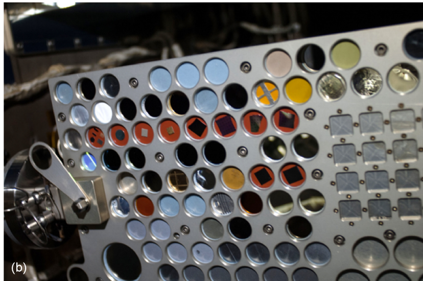
Figure 9.—MISSE 8 PEC and ORMatE-III on the ISS ELC-2. (a) During the STS-135 shuttle mission in July 2011 shortly after deployment of ORMatE-III. (b) On-orbit image of the ram surface of ORMatE-III in July 2013.
