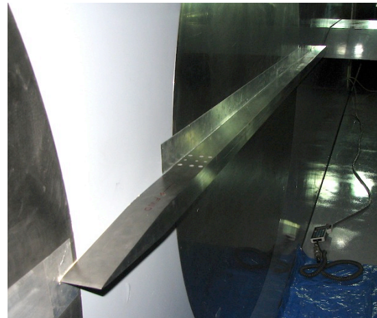
Figure 17. Photograph of 2-in. rail mounted on 9x7 WT aft window blank
