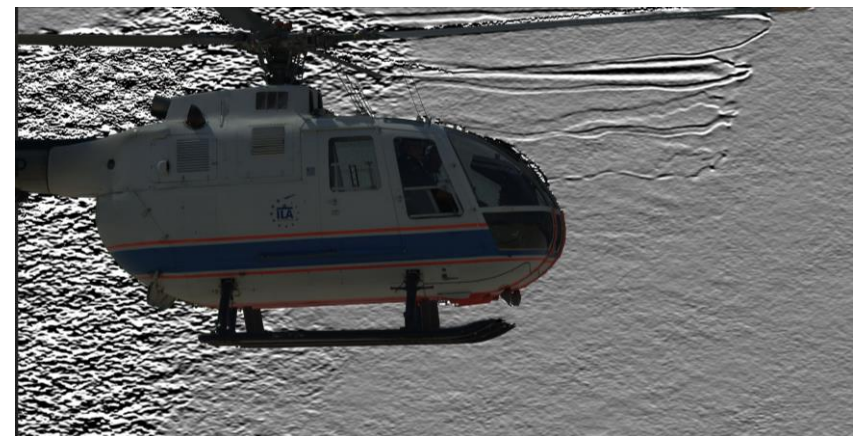
RBOS of a BO-105 in slow forward flight Raffel et. al. , DLR Goettingen
