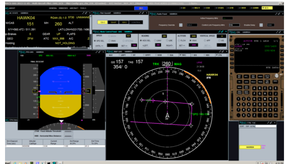
Figure 3. MACS Pseudo Pilot Displays. The Pseudo Pilot displays handle multiple aircraft and allow for basic maneuvering.
