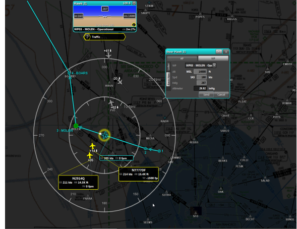
Figure 4. VSCS Traffic Display. The display shows a centered ownship, with proximal traffic and advisories.
