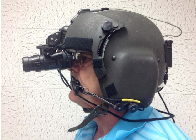
Figure 8. Night Vision Goggles (NVGs) mounted to pilots' helmet.
