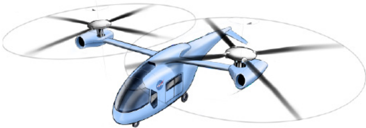
Figure 3: Side-by-Side (Lateral-Twin) Air Vehicle
