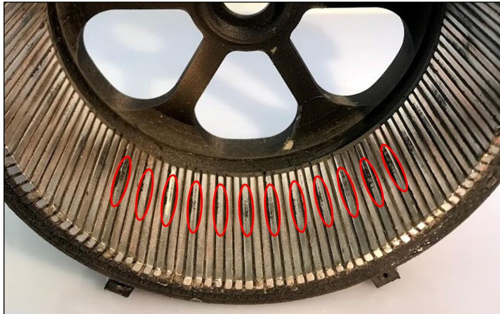
Modulator and Ring Gear Rubbing Visible from Black Marking Compound
