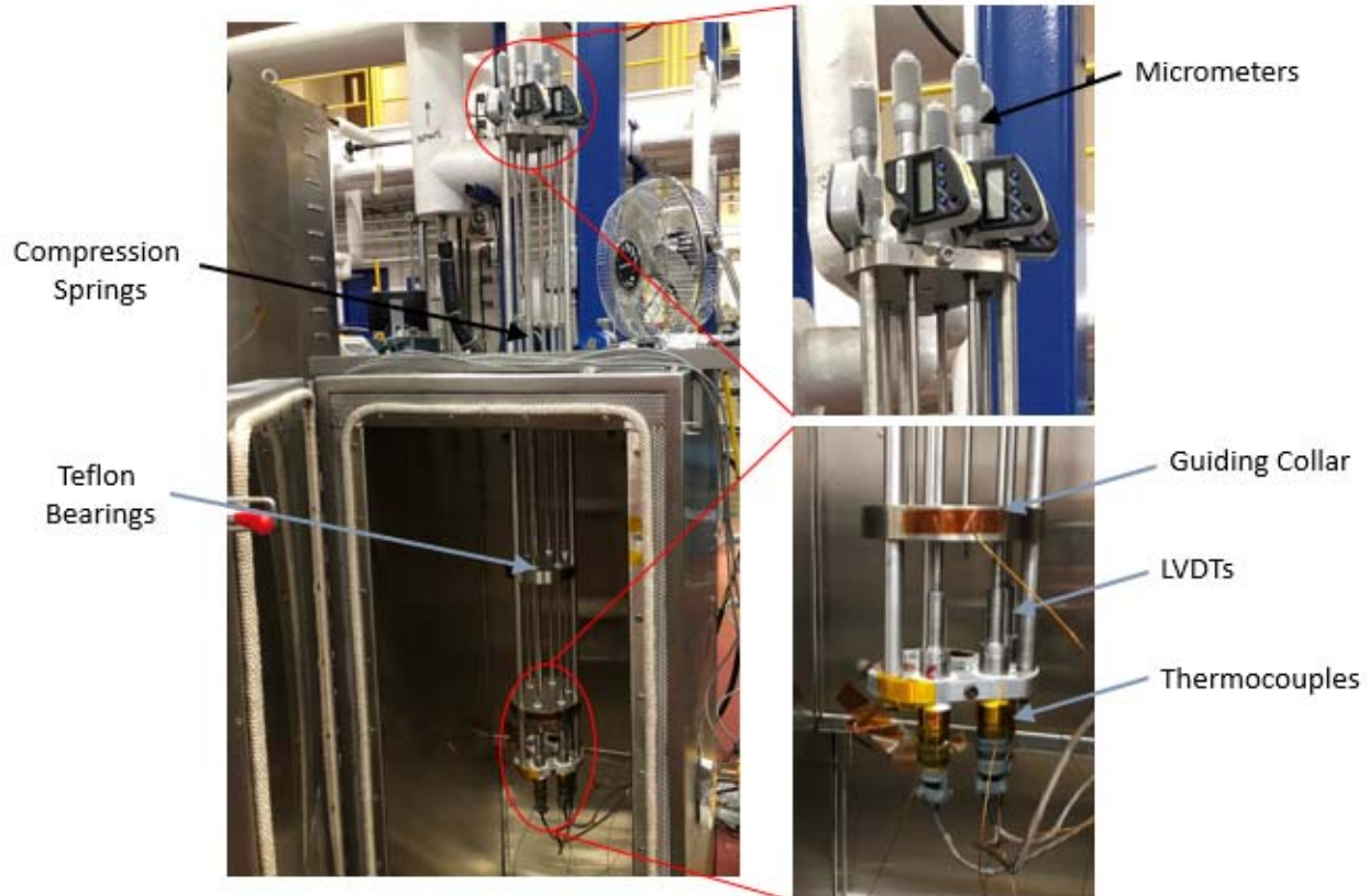
Figure 5. LVDT Calibration System.
