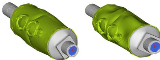
Figure 22. Analysis Results Showing Surface Distortions: before Applying Torque (left) and after Applying Torque (right).
