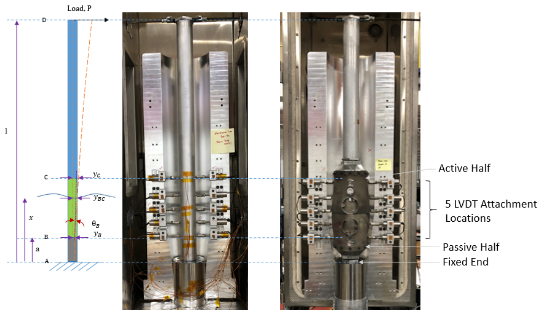
Figure 12. Bending Test Setup for Idealized Test (Left), Validation Specimen (Center) and Joint Specimen (Right).
