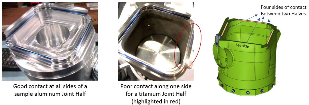
Figure 3. Variation at Contact Surfaces between Joints shown through Blue Layout Aid.
