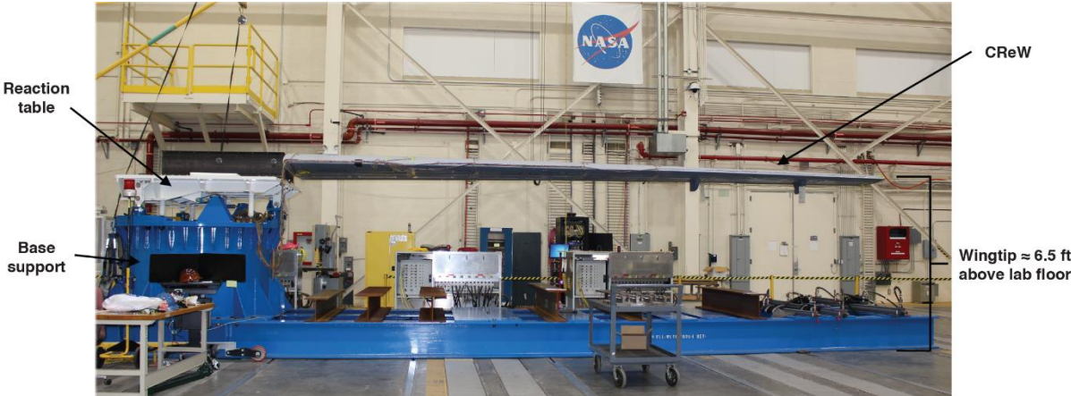
Figure 6: Modal test setup with CREW mounted on the WLF with wingtip \approx 6.5 ft above lab floor.
