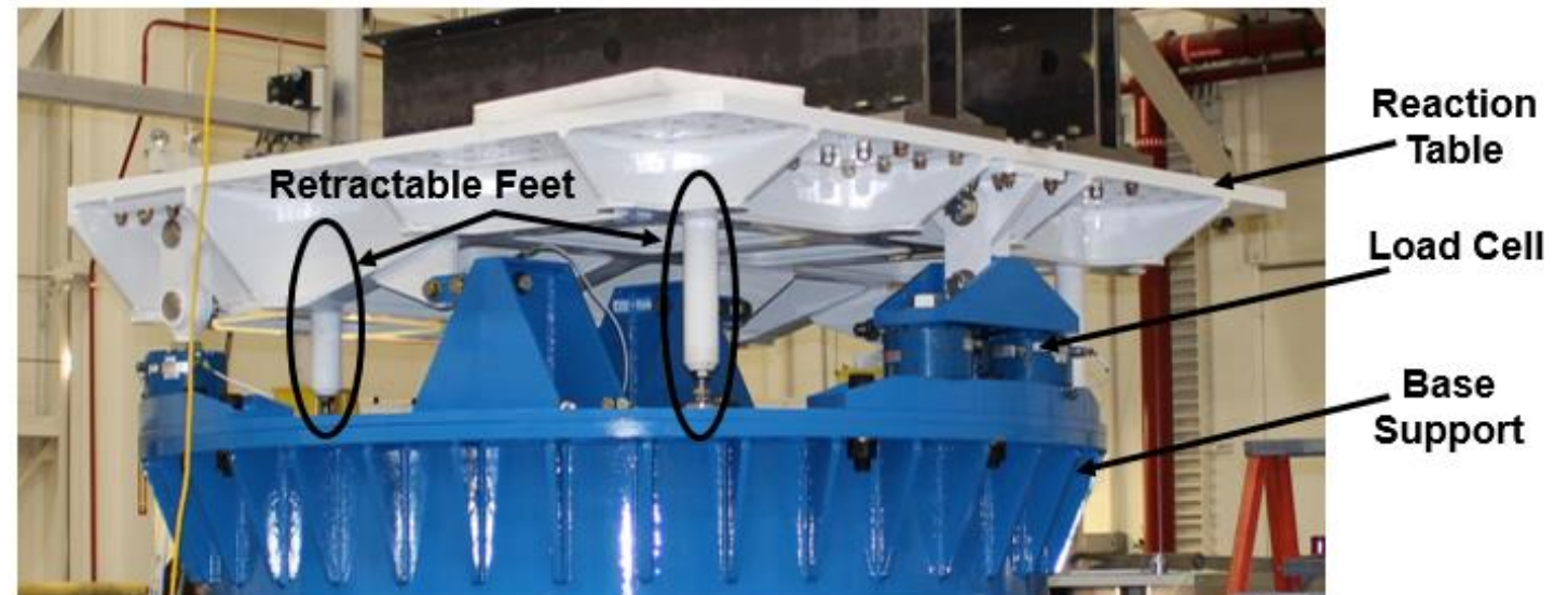
WLTF Reaction Table Supported with 4 Retractable Feet & 7 Load Cells
