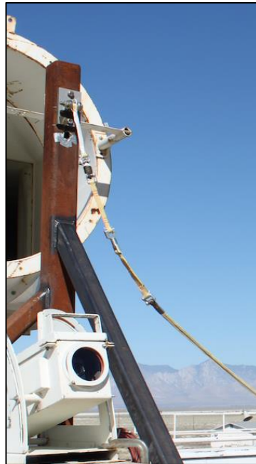
Fig. 11 Riser load measurement and sting attachment photo, with boresight camera.
