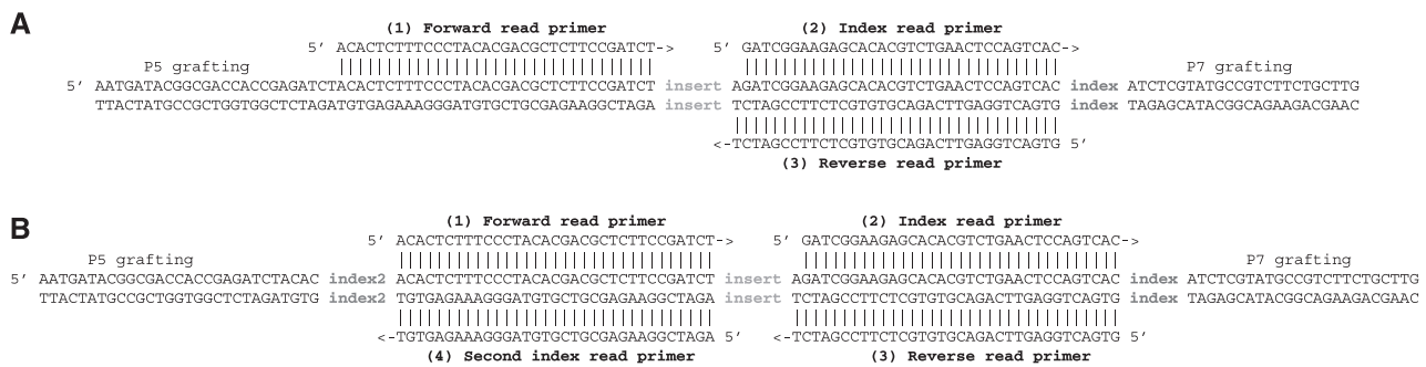
Figure 1. (A) Regular Illumina multiplex library design. The grafting sequences (P5 and P7) are used for template immobilization and amplification. Three distinct sequence reads (forward read, index read, reverse read) are primed from different adapter sites. (B) Double-index library design with an additional index incorporated into the second adapter. Here, four distinct sequence reads are performed.
