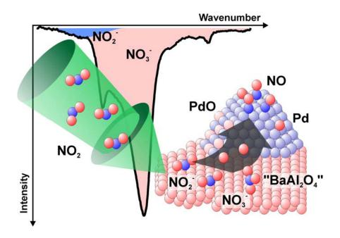
Nitrite formation during the initial stages of  $NO_x$  uptake on a nitrogen storage and reduction (NSR) catalyst is critically controlled by the interaction between the barium based  $NO_x$  storage material and the supported noble metal nanoparticles. This effect is due to reverse spillover of activated oxygen species, as demonstrated by molecular beam techniques and time-resolved IR surface spectroscopy on a NSR model catalyst.
