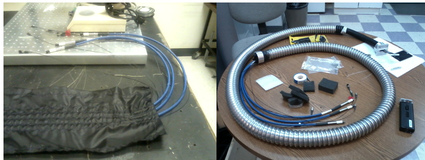
Figure 3.7: Left image: Top end of silk sheath with bundles. Right image: Sheath and bundles inside incompressible tube.
