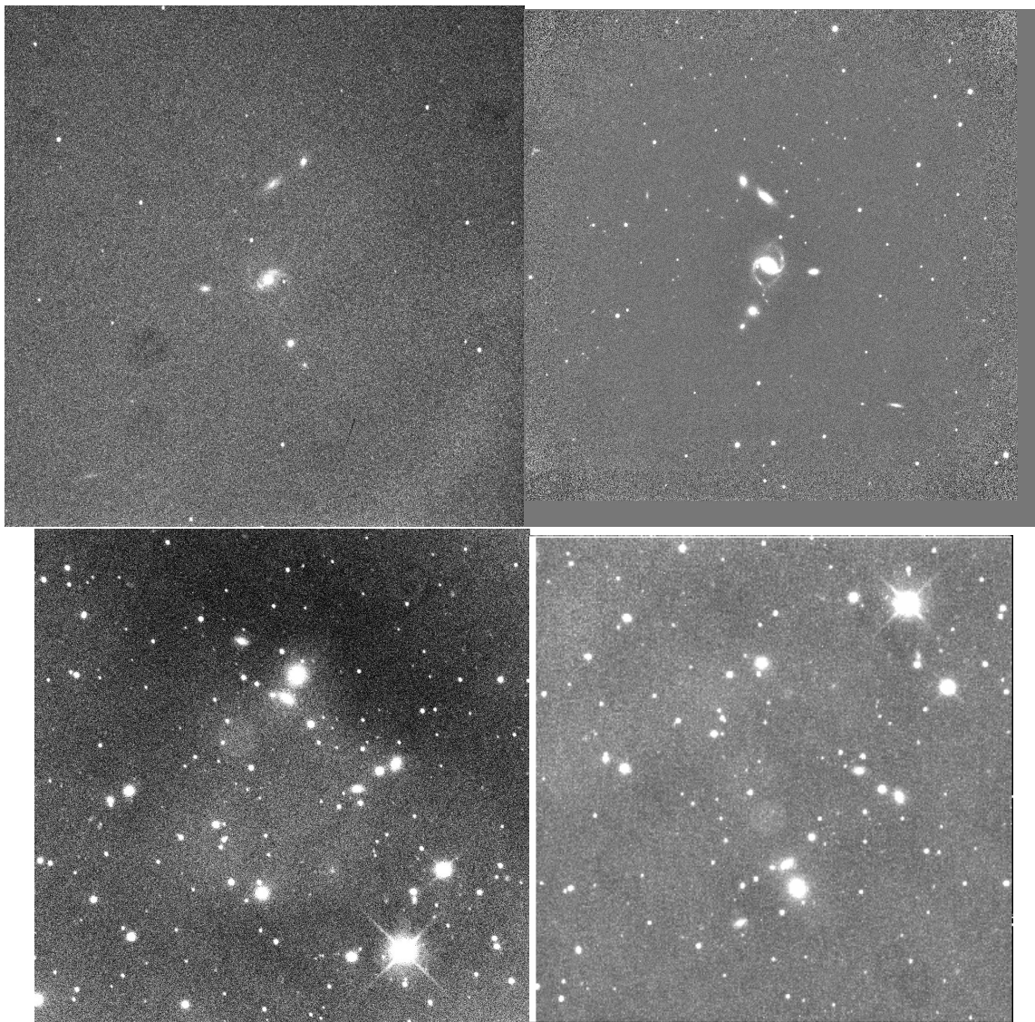
Figure 5.3: Examples of stacked PROMPT images. The left images are a single bias subtracted and flat fielded image and the images on the right are stacked. The top two images are for SCG15 and use the dithering method to remove the sky background. The bottom two images are for SCG68 and use SExtractor.
