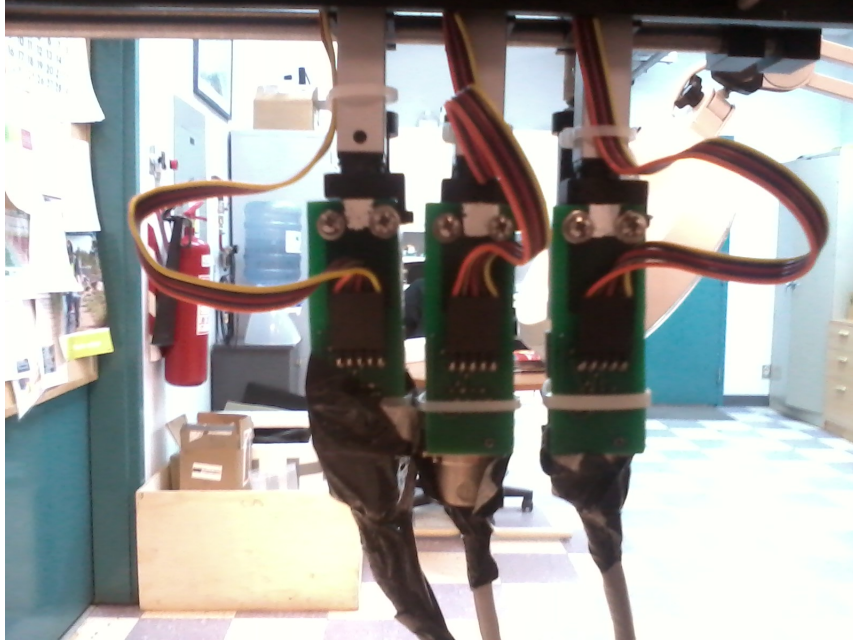
Figure 3.11: Probe entrance indicated on back of circuit board with white out.
