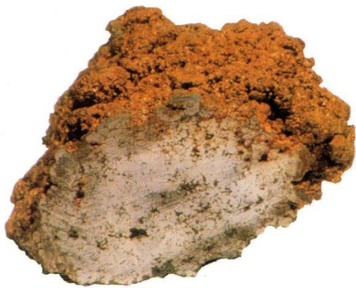
6 Section through a piece of bloom iron. Magnification approximately \times 1.2
