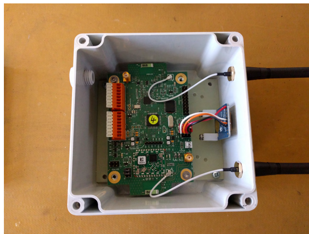
FIGURE 10. Hardware configured in a repeater node (RN) prototype.
