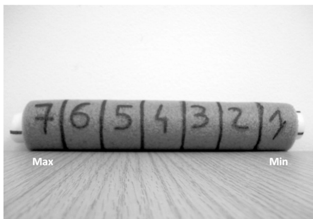
Figure 2 Device for grading skin tonicity. The tubular device is filled with layers of foam of increasing density in order to reproduce variations in skin tonicity, on a scale ranging from 1 “minimum firmness” to 7 “maximum firmness.” Grading is performed by comparing the resistance of skin versus the resistance of this dedicated foam-like device, when applying a constant pressure with fingers. The repeatability and reproducibility of the procedure has been validated by applying analysis of variance.
