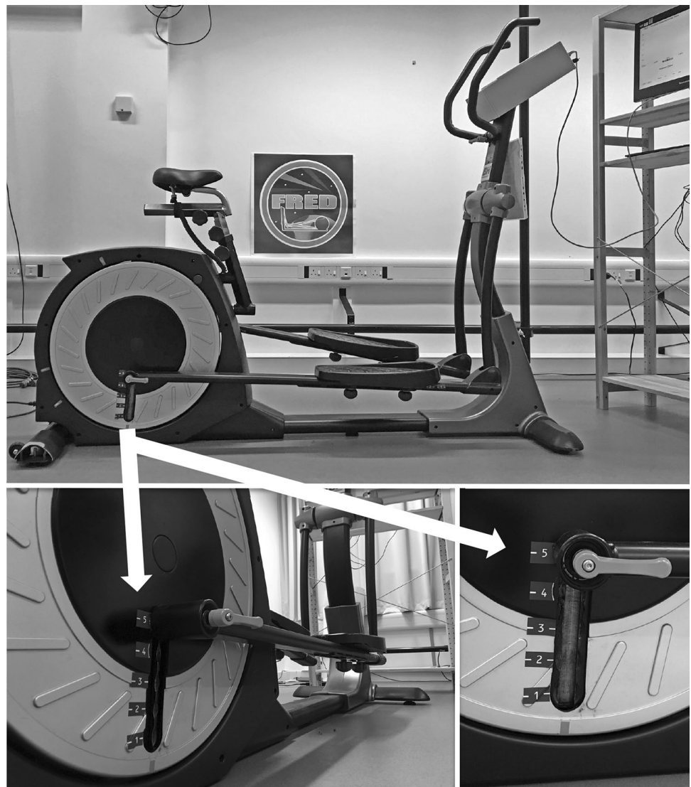
Fig. 1 FRED ( top ) and a close up view of the adjustable amplitude crank with the various amplitude settings (1–5) ( bottom left and right ). The crank location is highlighted with a white arrow
