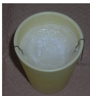
Figure 77. Crucible filled with the solution after the experiment. The Pt-wires of the baffle are visible.
