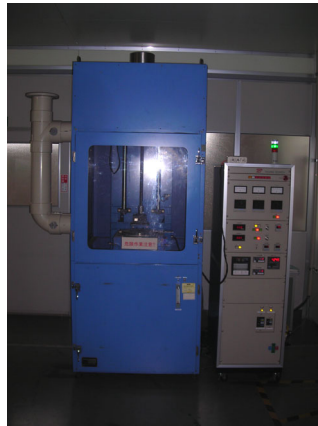
Figure 73. LPE machine from Techno search.
