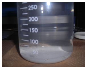
Figure 66. The doped ZnO is deposited at the bottom of the glassbeaker.
