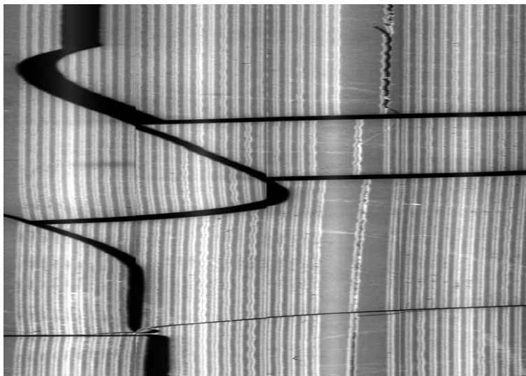
Figure 4.6: This acquisition has been performed on a disc with shrinkage of the recording layer. The black cracks are the visible part of the aluminium plate. At some cracks, the grooves (in white) present important shifts from one piece to the next.
