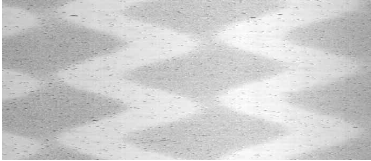
Figure 4.7: Magnified view of a film: the small dark spots are the pepper fog spots. This picture has been taken with a very low exposure time. Thus we can also see the pepper fog spots in the exposed areas of the film and see that these spots are uniformly distributed over the light and dark areas of the picture.
