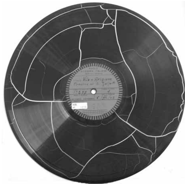
Figure 2.6: Acetate record with shrinkage of the recording layer: the aluminum base layer is visible at many places (white cracks).
