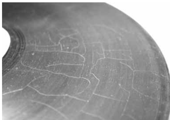
Figure 8.20: Audible sound could be extracted from this record, which shows limited shrinkage of the recording layer.
