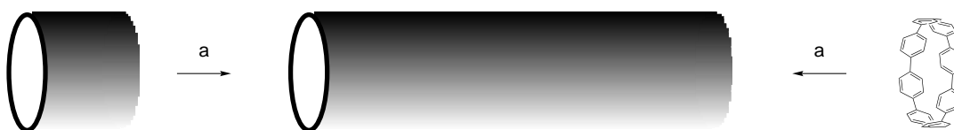
Figure 5.3: Strategies for synthesizing CNT from short cut carbon nanotubes (left) or [0_n] paracyclophane (right) template. a) iron precursor, DIBAH, 0.5 bars acetylene, benzene, rt.
