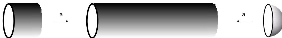
Figure 11.1: Strategies for synthesizing CNT from short cut carbon nanotube (left) or decapitated fullerenes (right) template. a) iron(0), DIBAH, 0.5 bars acetylene, benzene, rt.
