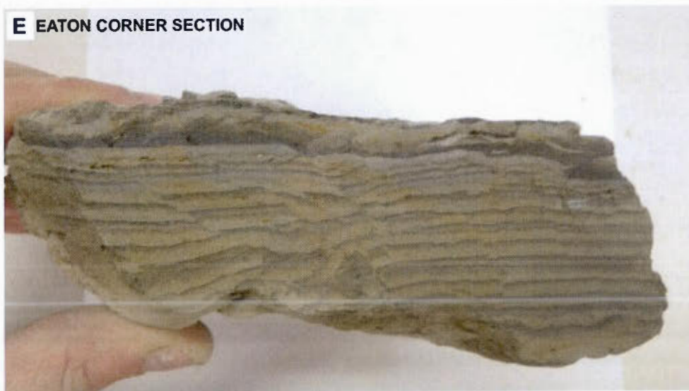
Figure 4.5 Fine-grained laminated sediment of the Saint-François and Chaudière watersheds: A: Missisquoi River probable varves; B: Ditton River probable varves; C: Ascot River probable varves (type-section); D: Moe River probable varves; E: Eaton Corner probable varves with high-angle reverse faulting with little deformation.
