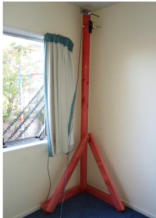
Figure 9: Potentiometer and manual dial gauge supported by timber props nailed to floor, Wairoa St Photo: D. Yeoh
