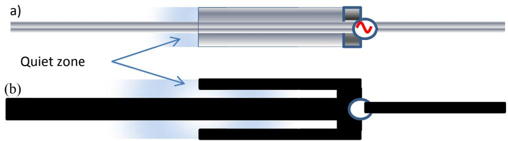
Fig 1-14(a) Cylinder and (b) planar choke analogue showing the self-choke function
