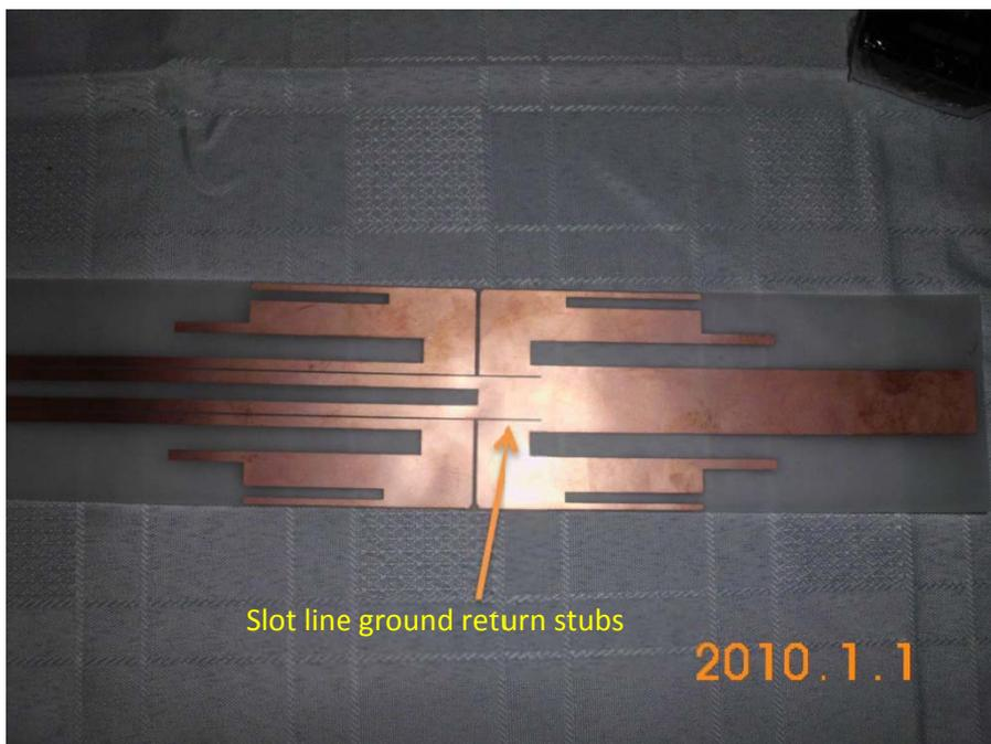
Fig 5-8 close-up of top element
