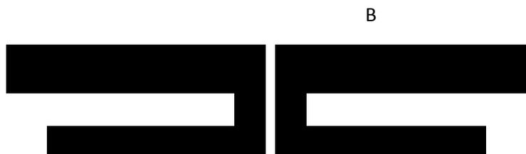
Arrangement for 22% bandwidth symmetrical radiation
