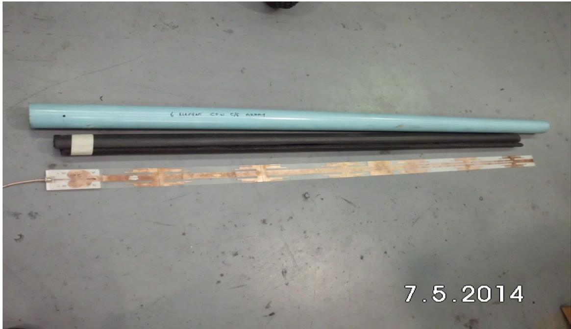
Fig 5-5 The full length of the "Coplanar waveguide (CPW)" array
