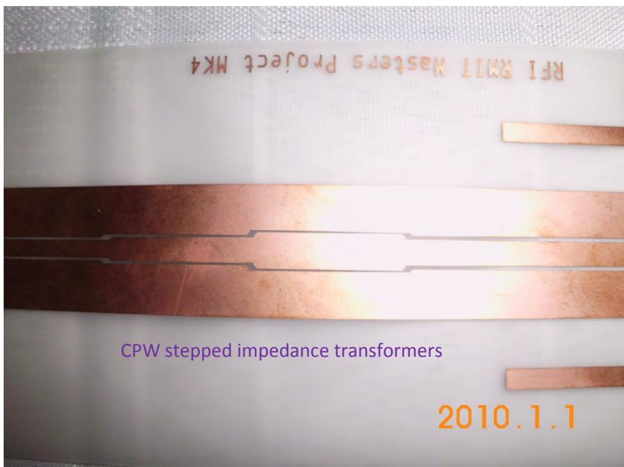
Fig 5-6 close-up of "Coplanar waveguide (CPW)" transmission line
