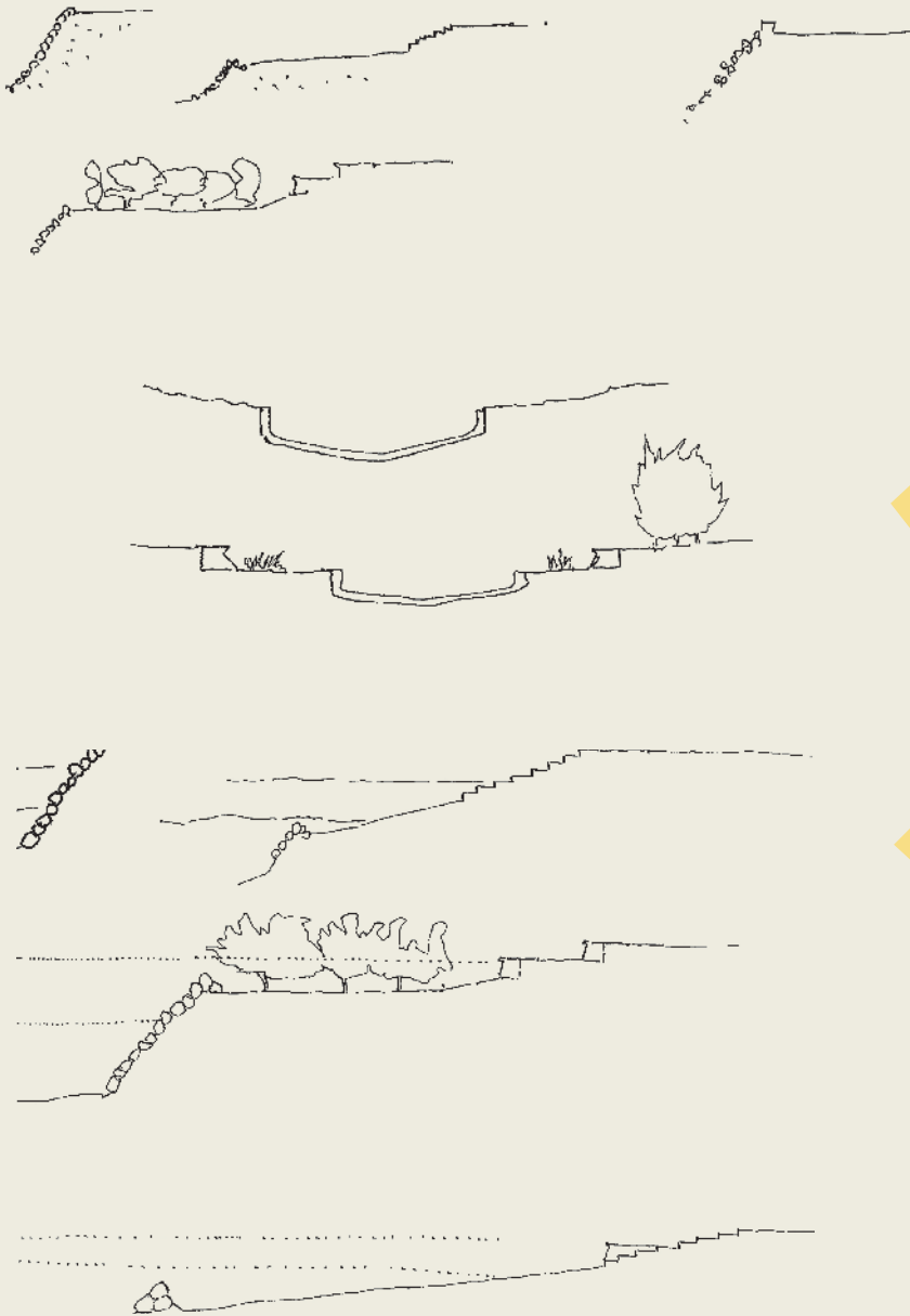
Different profiles were explored to engage with tidal flow and to encourage salt marsh species and mangroves, both of which grow in very specific tidal ranges.
