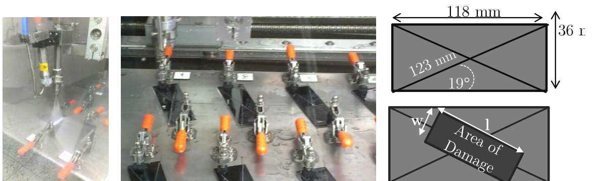
Figure 4.9: Steam Jet Test
